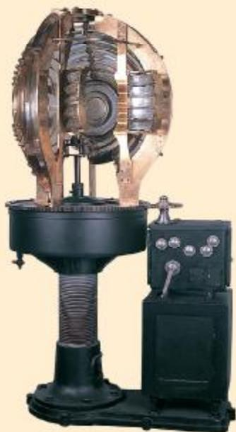
**Nº: 05. CONJUNTO DE APARATO ÓPTICO GIRATORIO PARA FARO ELÉCTRICO / NÚM: 05. CONJUNT D'APARELL ÒPTIC GIRATORI PER A FAR ELÈCTRIC / NO. 5. REVOLVING OPTICAL APPARATUS FOR AN ELECTR C LIGH-HOUSE**
